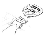
**Cyclometer 40 Installation.** Slide the Cyclometer into the mount bracket from front to rear until it snaps on. Choose the speed function, then spin the front wheel and watch for a reading. If the display remains at zero make sure that the receiver and transmitter are aligned and nearly touching.
