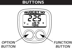
Function button is on the right. Press it to move in a loop sequence from one function to another.
